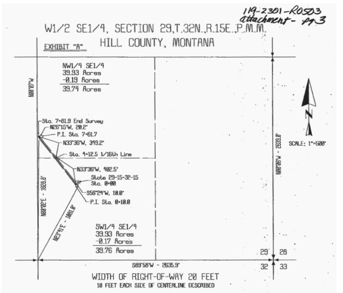
NOTES: 1. SURVEY STATIONS SHOWN ARE HORIZONTAL CHAINING STATIONS. 2. BASIS OF BEARINGS - GEODEDIC NORTH USING RTK GPS
