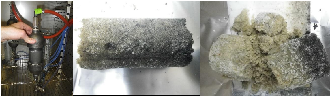
Figure 2. 2"x4" reactor system (left), cemented sand column with the presence of organics (middle), crumbled sand column where precipitation was promoted without organics (right).
