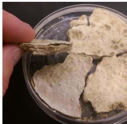
Figure 4. A whitish cap was observed to form on the surface of the ash material after treatment with biomineralization promoting solutions.
