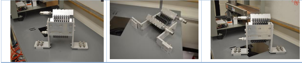
Figure 2-2. Machined aluminum parts of the manifold with 32 airjet valves attached.
