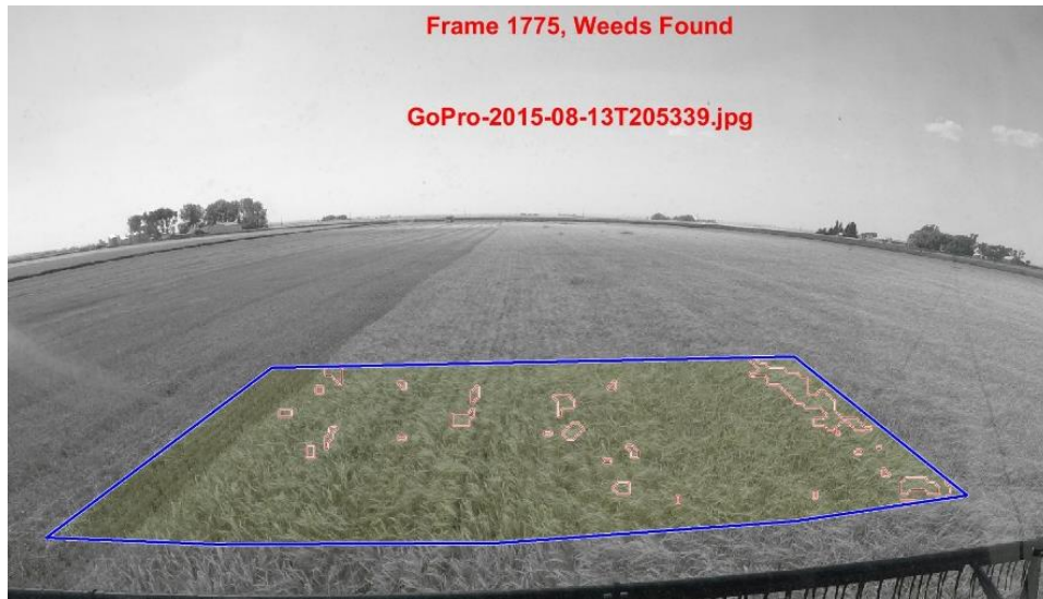
Figure 1-2. False detection of weeds in a GoPro image due to lighting change.
