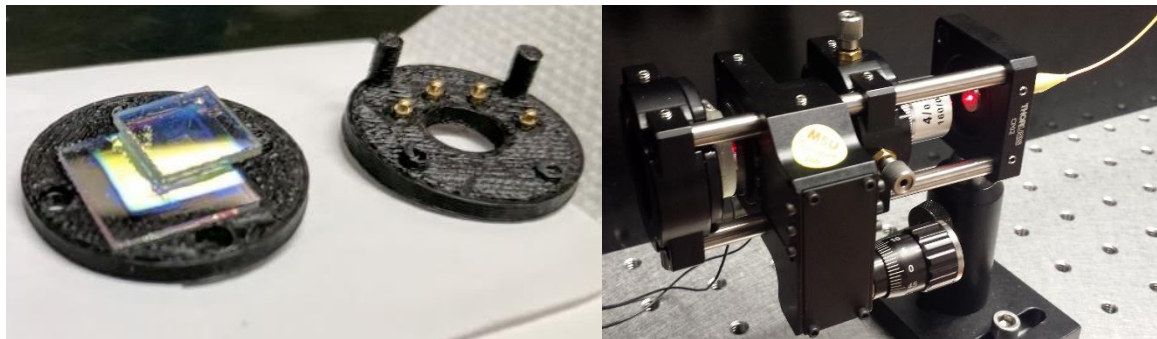
Figure 5-4 (Left) Compact holder for the LCAM with spring loaded electric contacts. (Right) Characterization setup for the LCAM.
