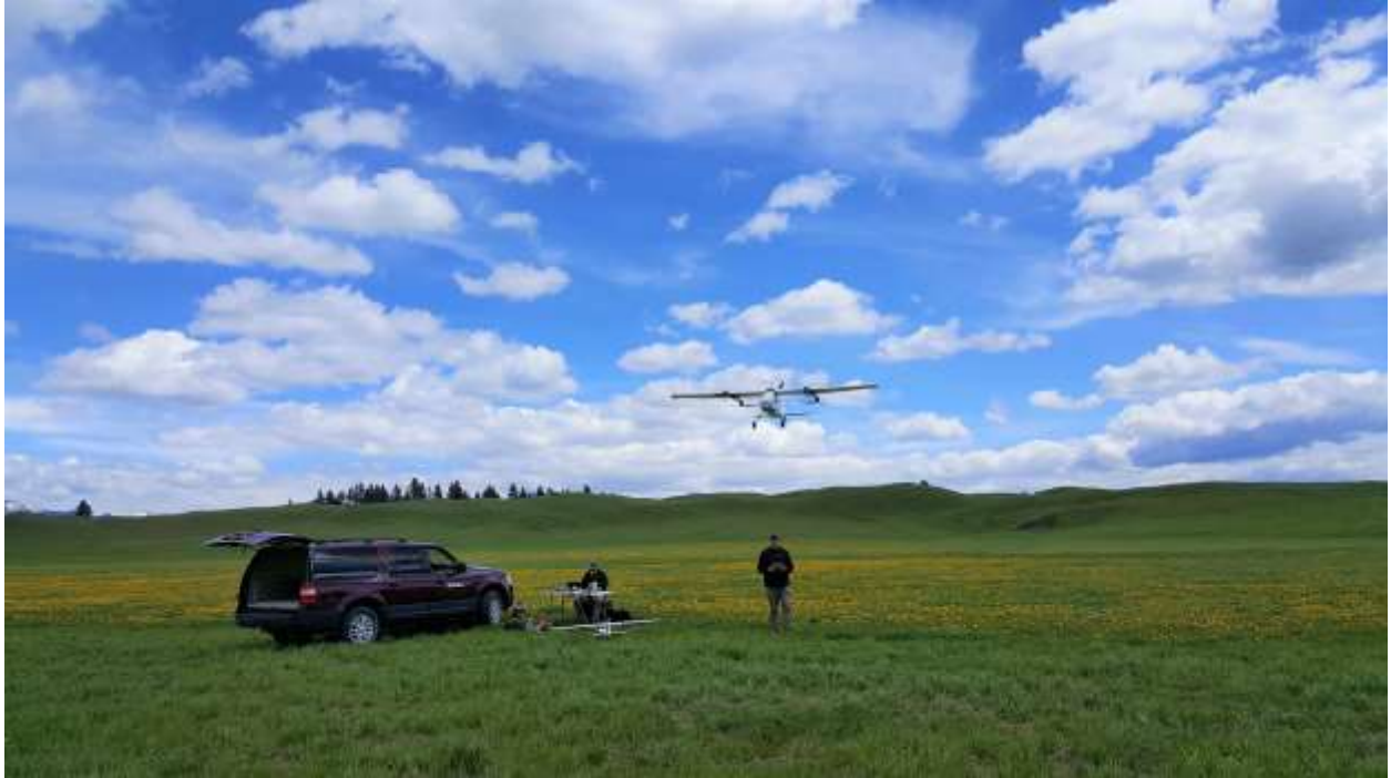
Testing the vertol Quadranger transition from hover to forward flight at UM's Bandy Ranch near Ovando, MT
