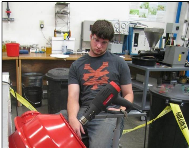
Figure 5. Garth Webster monitoring camelina seed conditioning operations using a cement mixer and hot air gun.
