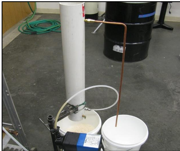
Figure 6. Student developed and built salt dryer for biofuels including pump and contacting vessel.
